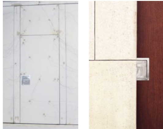
In order to ascertain the fire resistance class, a Variflex EI 30 wall with an integrated pass door was directly subjected to fire for over 30 minutes in a test lab.
